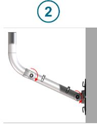
3. Attach the Outdoor Receiver/Mounting Bracket Assembly on the support arm.
